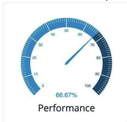
Figure 4.8: Performance Gauge gets its input from batch selection and seconds per unit which is selected by the user. The value from total counts is also used and obtained directly from Quality Gauge.
