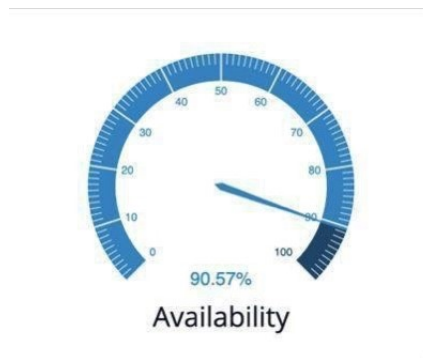
Figure 4.6: Availability Gauge depends on the batch selection table (which is an input from the user) and the Event Browser which is set up automatically. In addition, the events that are part of the production time must be defined and marked as "running" in the translation module.
